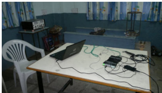
FFT connected to impact hammer, laptop & Accelerometer.
