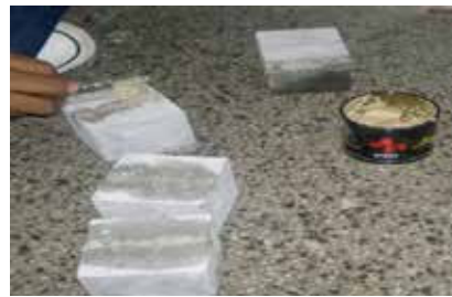
Fig 2.1.2 Inserting bacteria in to cracks
