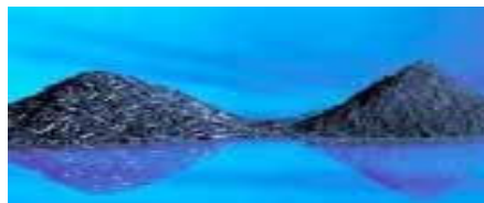
Figure 8: Granular Activated Carbon
