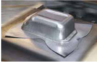
Fig.1.2- Figure for representation of a Deep Draw operation
