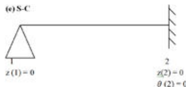
Figure 20: SS-Fix End condition
