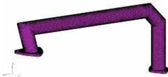
Fig-02: FEA model of pipe
