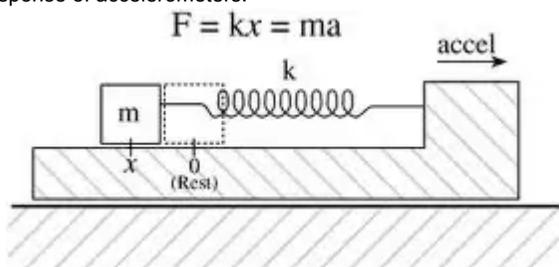
**Effect of Tilt in Accelerometer:**
