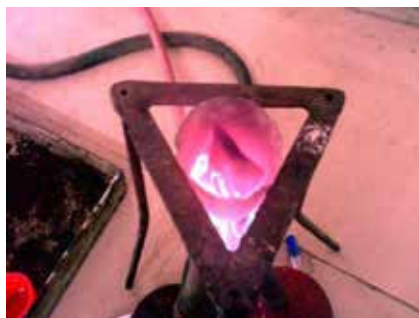
Fig.3 Burn process of substances in platinum vessel at temperature of 700-800°C.
