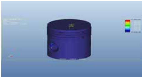
Figure 5: Final Solid Model of the Piston from RE Figure 6 : stress von Mises (WCS) Red color means critically stressed region Blue color means low stress region
