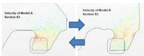
Figure 15: Reduced pressure drop by section Improvement
