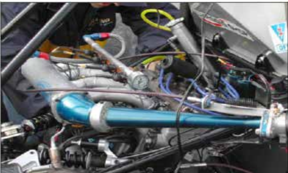
Figure 5: Inlet Manifold Type: Side Intake Concept
