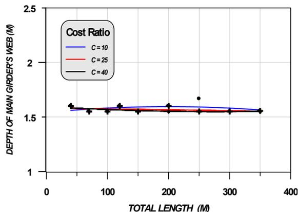
FIG. 14 Relation between total length and depth of main girder's web for  $F_y=248$  for steel and Bridge's Width =10 m.
