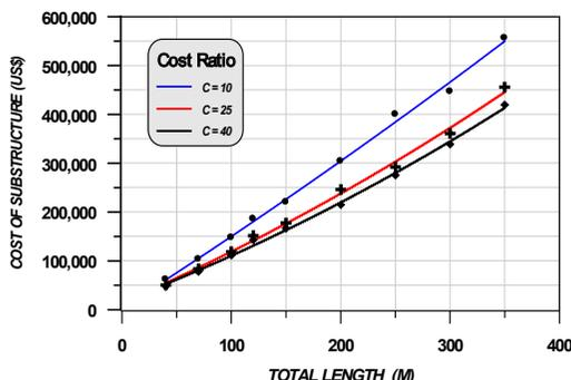
FIG. 7 Relation between total length and substructure cost for  $F_y=248$  for steel and Bridge's Width =10 m.
