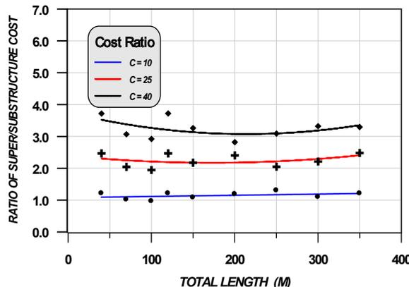
FIG. 9 Relation between total length and super/ substructure cost for  $F_y=248$  for steel and Bridge's Width =10 m.
