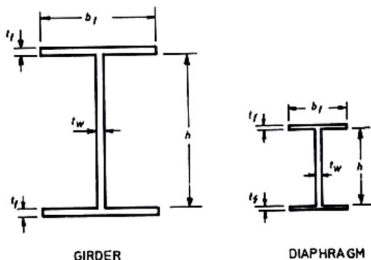
FIG. 2 TYPICAL SYMBOLS FOR STEEL SECTIONS OF GIRDERS AND DIAPHRAGMS.
