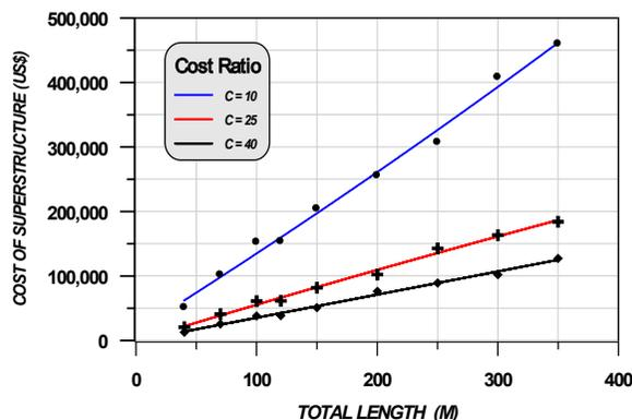
FIG. 8 Relation between total length and superstructure cost for  $F_y=248$  for steel and Bridge's Width =10 m.
