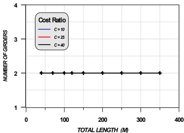
FIG. 11 Relation between total length and number of girders for  $F_y=248$  for steel and Bridge's Width =10 m.
