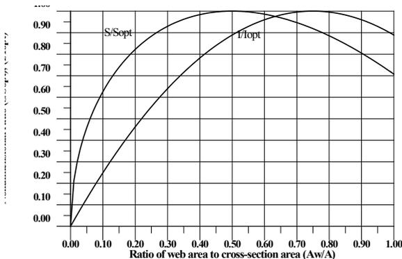
FIG. 1 OPTIMUM RELATIONSHIPS FOR MOMENT OF INERTIA AND SECTION MODULUS
