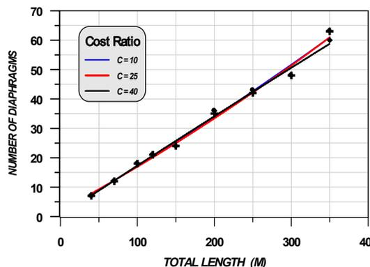
FIG. 10 Relation between total length and number of diaphragms for  $F_y=248$  for steel and Bridge's Width =10 m.
