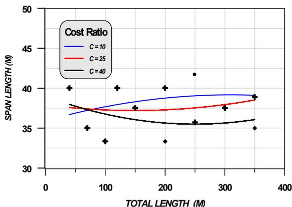
FIG. 12 Relation between total length and span length for  $F_y=248$  for steel and Bridge's Width =10 m.
