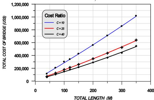
FIG. 6 Relation between total length and total cost for  $F_y=248$  for steel and Bridge's Width =10 m.
