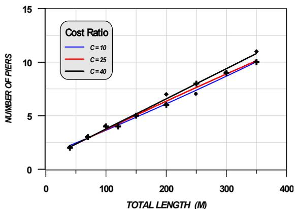
FIG. 13 Relation between total length and number of piers for  $F_y=248$  for steel and Bridge's Width =10 m.
