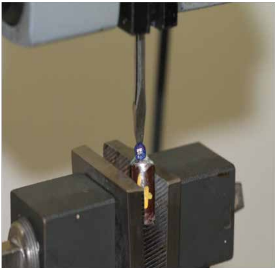
Fig 10. The sample teeth on the metallic rings are then tested with an Instron™ Universal Testing machine to record any changes in the shear bond strength after being immersed in soft drinks.
