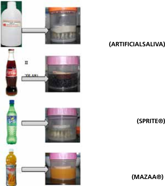
Fig 6. After bonding, the plaster slabs with sample teeth were submerged in different soft drinks for the regulat-
