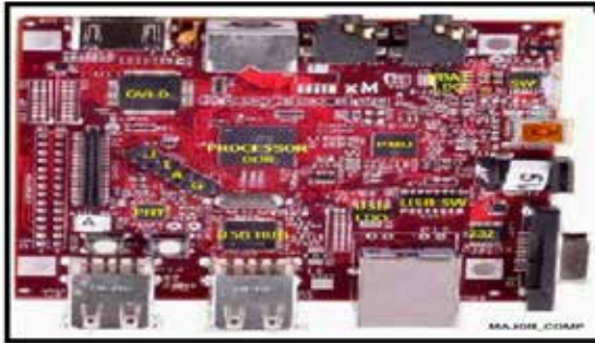
Figure 1: Beagle Board Major Components
