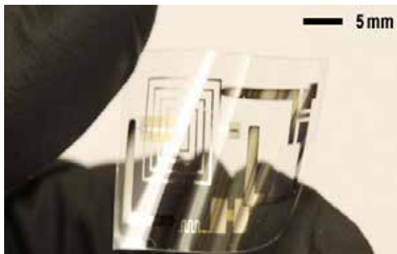
Fig.10 Edible Colpitts RF Oscillator(Courtesy ILLINOIS UNIV.)
