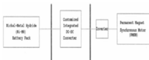
Figure 2. Power electronic circuit arrangement in HEVs.
