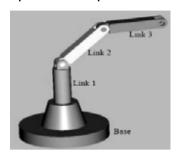
Mechanics of a manipulator can be represented as a kinematic chain of rigid bodies (links) connected by revolute or prismatic joints.
