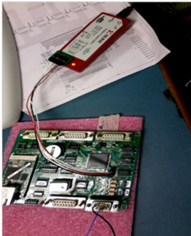
Illustration 10 Code for FPGA is dumped
