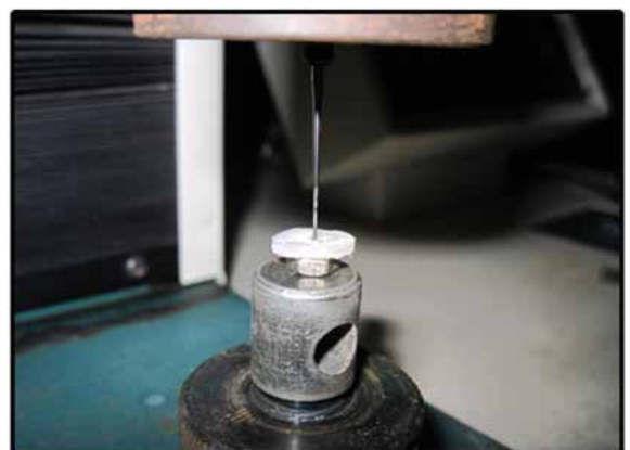
FIG 5: SECTION PLACED ON THE UNIVERSAL TESTING MACHINE FOR 'PUSH OUT TEST'
