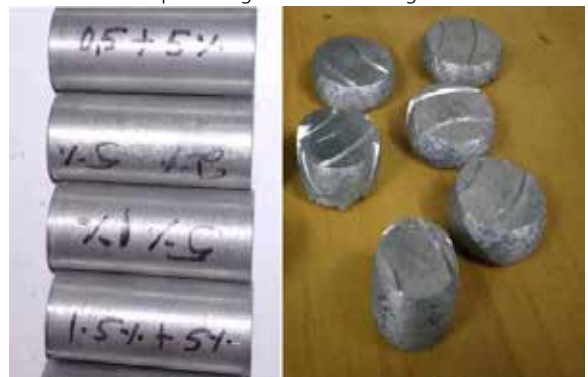
Figure:3. Compression test specimens (before and after testing)
