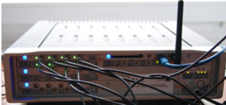
Figure 1: LMS SCADAS recorder used for data acquisition [2]
