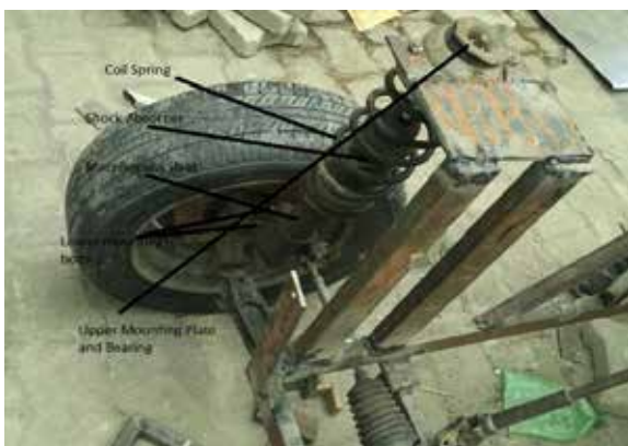
Figure: Macpherson Strut Suspension System
