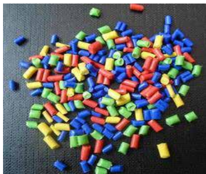
Fig-1 Waste plastics cut to required size The aggregate thus obtained were a mixture of angular and
