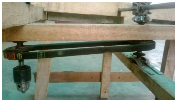
Figure 4: Drilling centre getting drive through bevel gear
