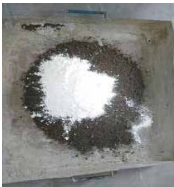
Fig. 1: Lime with Black Cotton soil
