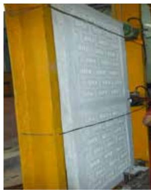
Figure 3. Schematic diagram showing 2D RC frame with brick infill
