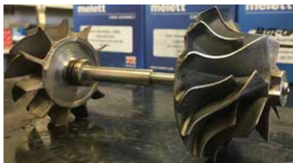
Figure 1: turbocharger shaft with turbine and compressor rotors [own source]
