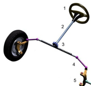
Fig: 1. Rack and pinion steering mechanism 1 Steering wheel; 2 Steering column; 3 Rack and pinion; 4 Tie rod; 5 Kingpin.
