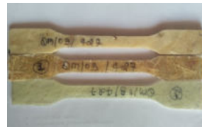
Fig 1: UTM (Universal Testing Machine) Fig 2: Specimen used for Tensile Strength Test
