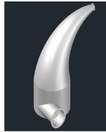
Fig 3. Circular cone cyclone separators
