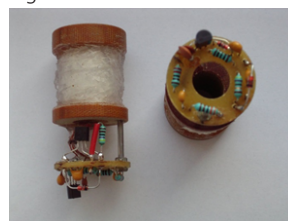
Figure 2: the coil sensor with the oscillator and temperature sensor
