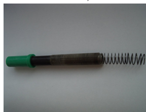
Figure 3: ferrite core with an outer piston as well as the glasstextite rod and a compression spring
