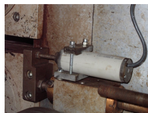
Figure 1: device with inductive sensor mounted on the left part of the adjusting mechanics of the machine
