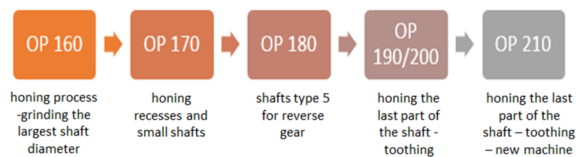
Figure 1: Production process of hard shafts
