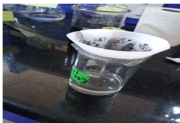
Fig: 3 Filtration Process after Adsorption process.
