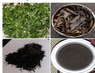
Fig: 1 Preparation of Neem Leaf Adsorbent
