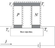
In Fig. 1 the schematic diagram of thermoelectric module is shown.
