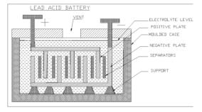
Fig. 3 Lead Acid Battery
