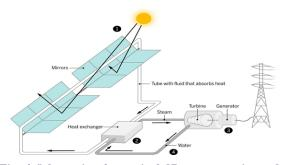
(Fig. 4 Schematic of a typical 1D concentrating solar thermal system.)
