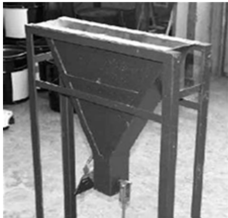
Fig.4 V-funnel Test of SCC
