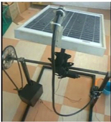
Fig 1: When light detected by LDRs at the centre, is more then it occupies centre position.
