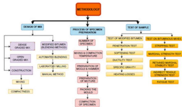
Figure 2: Material, Process and Testing involve the methodology for bitumen and polymer base road construction.
