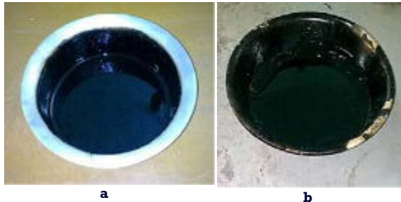
Figure 3: a) Bitumen, b) 10% Waste Plastic
