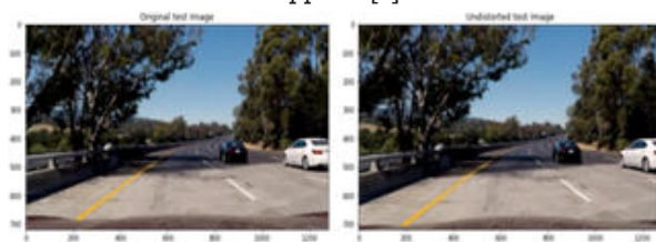
Figure 6: Before and after results of un-distorting an example image (Source: Udacity)
