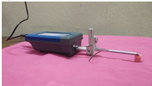
Figure 3: surface roughness testing with profilometer
