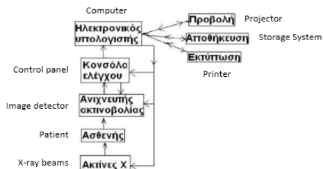
Figure 20. The structure of the digital radiographic system.
