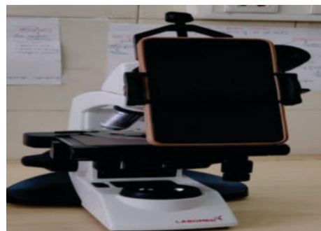
Fig 2 - Elephantboat Telescope Spotting Scope camera cell phone adapter mount kit attached to Labomed LX 400i
