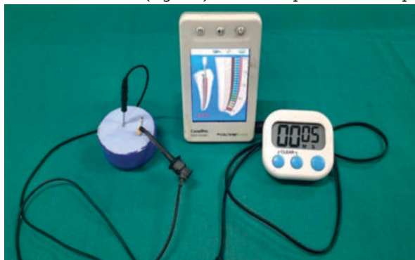
Figure 1 Experimental set-up of the in vitro alginate model for electronic working length measurement
