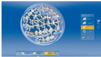
Figure 2. Restorations on a disc designed in inLab software (13)
