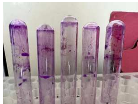
Fig.2: Biofilm adherence to glass test tube is shown by staining with 0.1% crystal violet
