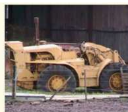
Loader without roll over protection. Photo: J.Culvenor
