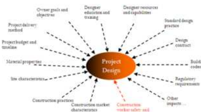
Fig. 2. Parameters which impacts a project's design
