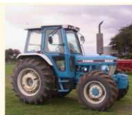
Cab and integrated roll over protection. Photo: J.Culvenor
