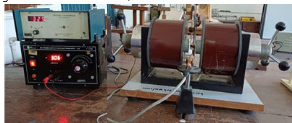
Fig 1. Hall experiment instrument set up used for the study of effect of EMF on in vitro pollen germination
